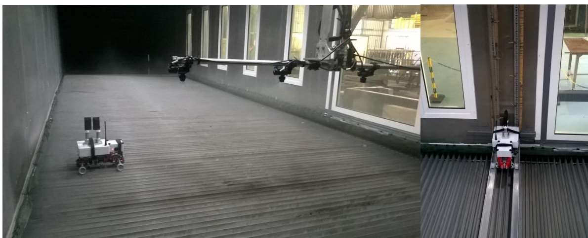
Figure 1: horizontal sampling protocol (left) and vertical sampling (right) in the wind tunnel.
