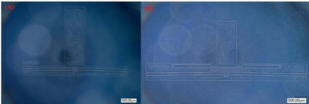
**Figure 4.** Photos of the fabricated Highly Nonlinear Curved Beam system (A) and Compensational Springs system (B). Note the difference in the footprint size.
