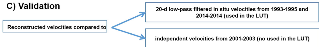
Figure 2. Schematics of the methodology used to obtain the cross-track reconstructed velocities ((a) construction of the look-up table (LUT), (b) mean surface velocity estimate, and (c) validation). CMEMS, Copernicus Marine and Environment Monitoring Service; MDT, mean dynamic topography; SLA, sea level anomaly.
