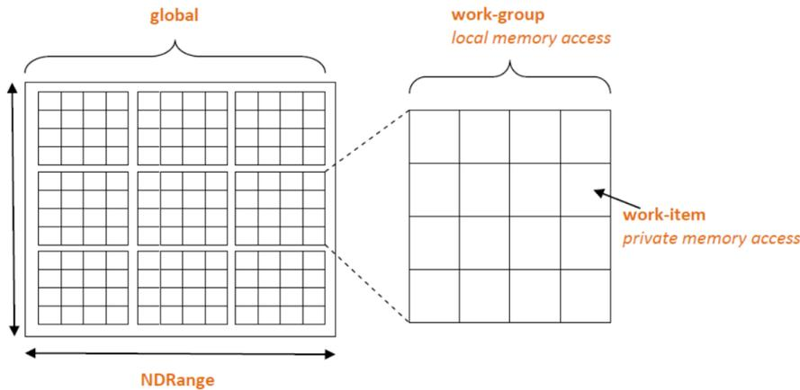
**Fig. 3** OpenCL two dimension mapping. Source : engcore.com
