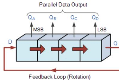
**Fig. 6** Shift-Register Pattern - Ring counter. Source : electronics-tutorials.ws
