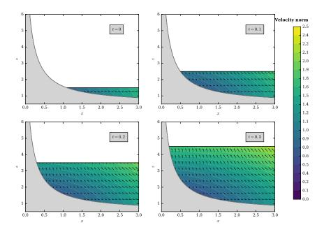
FIGURE 8. Decreasing bathymetry in 1/x: velocity norm and vectors at  $t=0,\ 0.1,\ 0.2$  and 0.3 s in (x,y=0,z) for the parameters set  $\alpha=1$  m.s,  $\beta=0.1$  m,  $b_0=-1$  m,  $t_0-t_1=2$  s,  $c_0=1.2$  m<sup>2</sup>.
