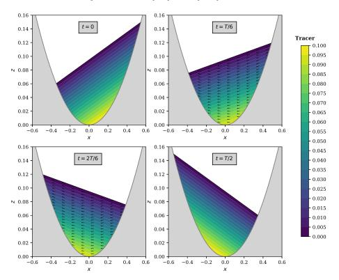
FIGURE 6. Analytical solution of radially-symmetrical parabolic bowl with variable density (see prop. 2): free surface, velocity vectors and tracer for t=0,T/6,2T/6,T/2, in (x,y=0,z) slice plane with the period T defined by  $T=2\pi/\omega$  and for parameters set to  $\eta=0.1$  m,  $h_0=0.1$  m,  $a=1, \alpha=1$  m<sup>-1</sup>, L=4 m.
