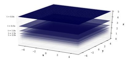
FIGURE 9. Draining of a tank: free surface every 0.5 s from initial time, for parameters set to  $\alpha = 5$  m.s,  $\beta = 0$  s<sup>-1</sup>,  $t_0 = 1$  s,  $t_1 = 1$  s and L = 10 m.
