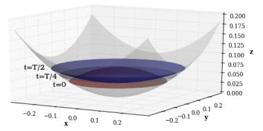
FIGURE 3. Analytic solution for 3D Axisymmetrical parabolic bowl (see prop 1): free surface at t=0 (red), t=T/4 (dark grey), t=T/2 (blue), with the period T defined by  $T=2\pi/\omega$  and for parameters set to  $h_0=1$  m,  $\alpha=2$  m<sup>-1</sup>,  $\beta=1$  m<sup>-1</sup>.s<sup>-1</sup>,  $\gamma=0.3$ , c=-1 s<sup>-4</sup>, L=1 m.
