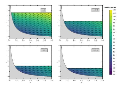
FIGURE 7. Analytical solution for hyperbolic topography (see prop 3): velocity norm and vectors at  $t=0,\ 0.05,\ 0.1$  and 0.15 s in (x,y=0,z) for parameters set to  $\alpha=0.5$  m.s,  $\beta=0.1$  m,  $b_0=0.4$  m,  $t_0-t_1=2$  s,  $c_0=1.2$  m<sup>2</sup>.
