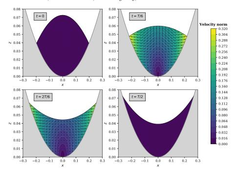
FIGURE 4. Analytic solution for 3D Axisymmetrical parabolic bowl (see prop 1): velocity field and norm at t=0,T/6,2T/6,T/2, in (x,y=0,z) slice plane with the period T defined by  $T=2\pi/\omega$  and for parameters set to  $h_0=1$  m,  $\alpha=2$  m<sup>-1</sup>,  $\beta=1$  m<sup>-1</sup>.s<sup>-1</sup>,  $\gamma=0.3$ , c=-1 s<sup>-4</sup>, L=1 m.
