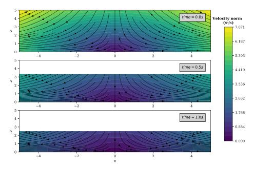
FIGURE 11. Draining of a tank (non-hydrostatic case): velocity norm and streamlines at t=0,0.5,1.0 s, in (x,y=0,z) slice plane for parameters set to  $\theta=0, \alpha=\text{m.s.}, t_1=1$  s,  $p^a=0 \text{ m}^{-2}.\text{s}^{-2}, z_b=0 \text{ m}$  and L=10 m.
