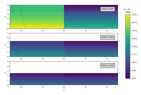
FIGURE 10. Analytical solution for the draining of a tank (see prop. 6: non-hydrostatic pressure (left, x < 0) and hydrostatic pressure (right x > 0), at t = 0, 0.5 and 1 s, in (x, y = 0, z) plane with parameters set to  $\gamma = 0$  s<sup>-1</sup>,  $\delta = 0$  m.s<sup>-1</sup>,  $\theta = 0$ ,  $\alpha = 5$  m.s,  $t_0 = 1$  s,  $t_1 = 1$  s,  $p^a = 0$  m<sup>2</sup>.s<sup>-2</sup>,  $z_b = 0$  m and L = 10 m. Dashed line represents pressure profile.
