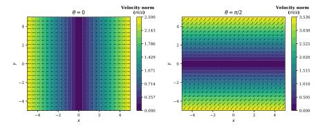
FIGURE 12. Draining of a tank (non-hydrostatic case): velocity norm and vectors at initial time in  $(x,y,z=h_0/2)$  slice plane with  $\alpha=5$  m.s,  $t_1=1$  s,  $p^a=0$  m $^2$ .s $^{-2}$ ,  $z_b=0$  m and L=10 m.
