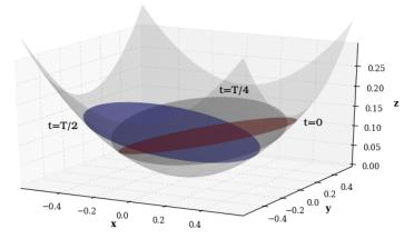
FIGURE 5. Analytical solution of radially-symmetrical parabolic bowl with variable density (see prop. 2), 3D planar surface: free surface at t=0 (red), t=T/4 (dark grey), t=T/2 (blue), with the period T defined by  $T = 2\pi/\omega$  and for parameters set to  $\eta = 0.1$  m,  $h_0 = 0.1$  m, a = 1,  $\alpha = 1 \text{ m}^{-1}, L = 4 \text{ m}.$
