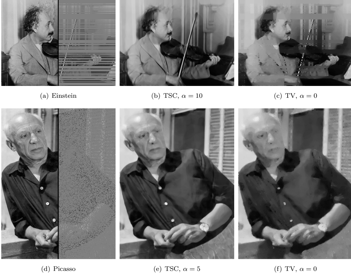
Figure 9: Image inpainting using the proposed curvature-based energies. (a) shows a blend of the original “Einstein” image with its degraded version where we have removed 80% of the lines. (d) shows a blend of the “Picasso” image with a version where we have removed 90% of the pixels. (b) is the inpainting result of the “Einstein” and (e) is the inpainting result of the “Picasso” image. For comparison, (c) and (f) show the result of standard TV regularization. Observe that our proposed curvature based regularization leads to significant better inpainting results.
