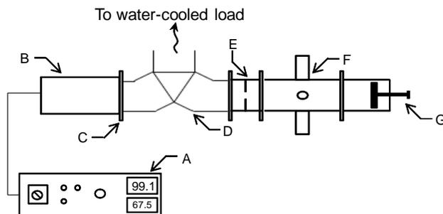
**Figure 1.** Schematic diagram of the microwave setup used in the study. (A) Variable power generator, (B) magnetron, (C) waveguide flange connector, (D) water-cooled circulator, (E) variable coupling aperture, (F) sample section, (G) plunge tuner.
