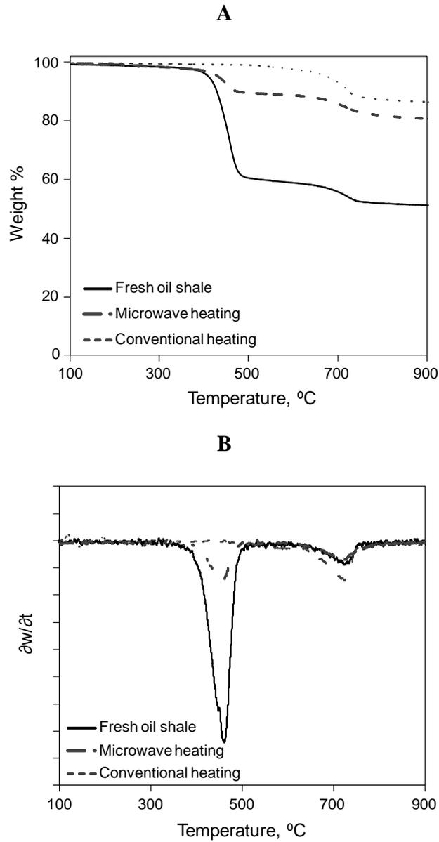
**Figure 4.** TGA of fresh and spent shale samples from decomposition under microwave irradiation and conventional heating, experiments under nitrogen flow (A); weight derivative in function of time (B).
