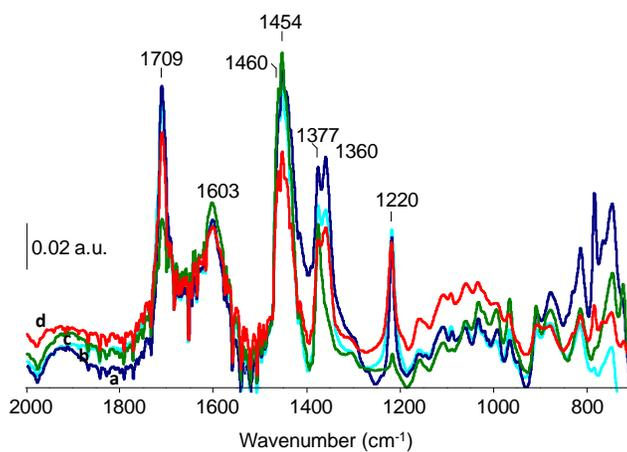
**Figure 10.** Normalized IR spectra in the  $\delta(\text{C-H})$  vibration region: a – microwave heating; b – conventional heating with BEA zeolite; c – conventional heating; d – microwave heating with BEA zeolite.
