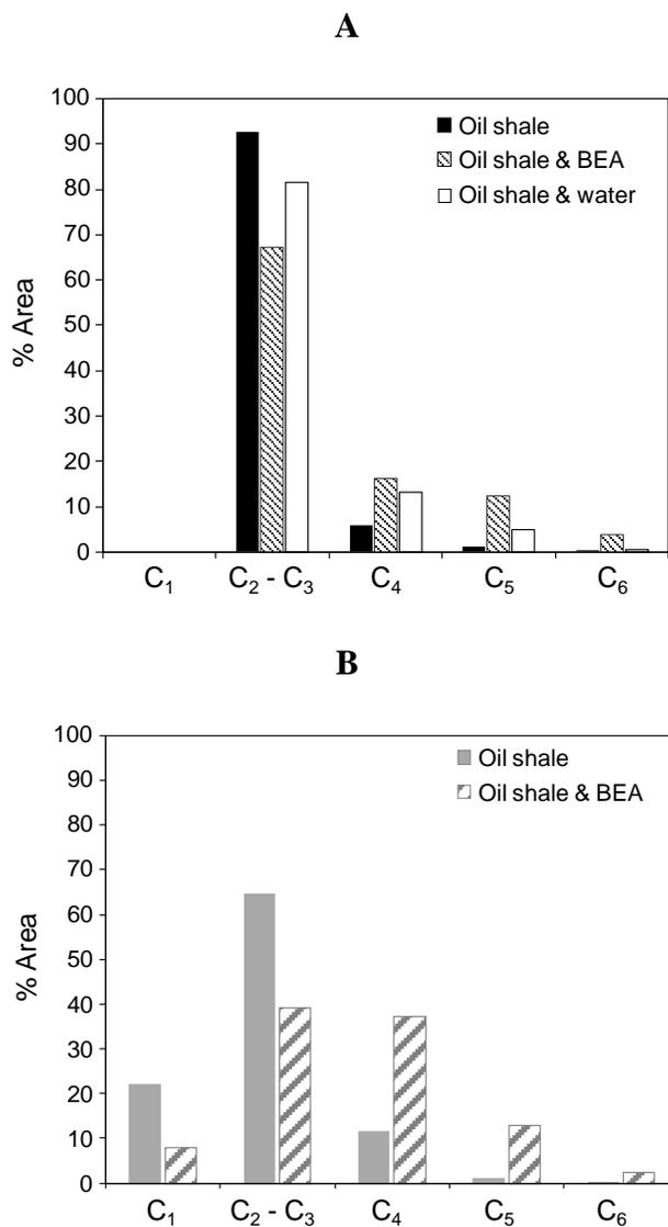
**Figure 8.**Result from peak integration of the GC-MS chromatogram for the gas samples obtained via microwave irradiation (A); peak integration of the chromatogram from GC of the gas samples obtained via conventional heating (B).
