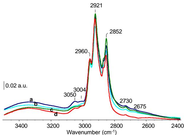
**Figure 9.** Normalized IR spectra in the  $\nu(\text{C-H})$  vibration region: a – microwave heating; b – conventional heating with BEA zeolite; c – conventional heating; d – microwave heating with BEA zeolite.
