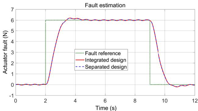
Fig. 6. Actuator fault estimation.
