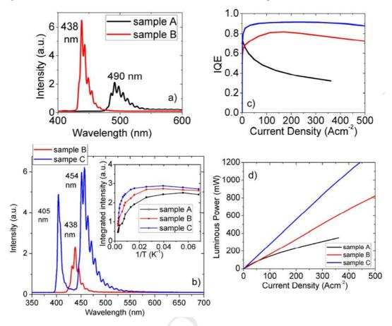
Fig. 3. Low temperature (15 K) PL spectra comparison of sample A and B (a) and sample B and C (b) (inset shows the integral PL intensity versus *1/T* for sample C). Calculated IQE (c) and luminous power (d) comparison of sample A, sample B and sample C.
