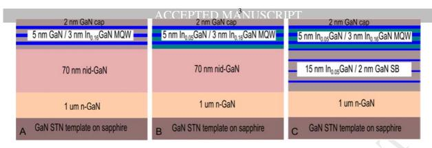
Fig. 1. Structure of the three samples under this study: reference sample A with GaN buffer and GaN barrier, reference sample B with GaN buffer and  $In_{0.05}Ga_{0.95}N$  barrier and final structure of sample C with semi-bulk  $In_{0.05}Ga_{0.95}N$  buffer and  $In_{0.05}Ga_{0.95}N$  barrier.
