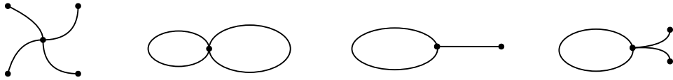
Figure 2: Respectively a star graph, a double-ring graph, a tadpole graph and a two-tails tadpole graph.
