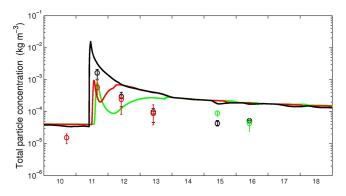
**Fig. 7.** Modelled (curve) and measured (circle) total inorganic particle concentration in DUST-meso at different depths on a logarithmic scale: 0 m (black), 5 m (red) and 10 m (green). Error bars show the total range of measured data.
