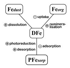
**Fig. 2.** Chemical model of iron. Processes supplying DFe haven a sign of + and those removing DFe a sign of -.
