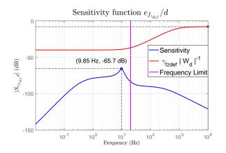
Fig. 5. Sensitivity function  $e_{f_{z_{def}}}/d$
