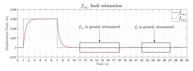
Fig. 10. Fault estimation result from 0 to 30 seconds
