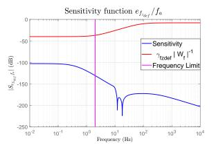
Fig. 6. Sensitivity function  $e_{f_{z_{def}}}/f_a$
