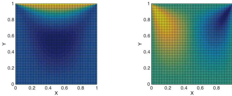
**Fig. 9** Driven cavity flow problem. Velocity field: (left) x-components and (right) y-component.
