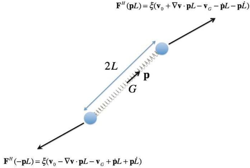
**Fig. 1** Extensible rod immersed in a flow.
