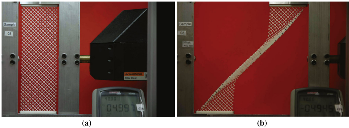
Fig. 32 a Reference configuration ( \lambda = 0 ), b damage onset ( \lambda = 0.976 ) of a shear test
