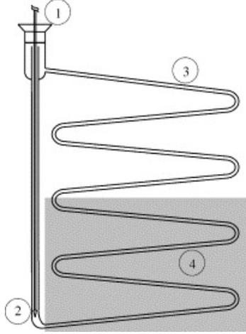
Figure 1: Scheme of the tubular loop reactor with air lift pump. (1) Gas inlet; (2) gas sparger (air+CO<sub>2</sub>); (3) illuminated part of the tubular reactor; (4) dark part of the tubular reactor [24].
