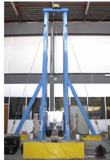
FIG. 4. ISAE-Supaero's existing drop tower structure. The tower features an electronically operated motor and pulley system for raising test materials and two low-friction rails for keeping the test materials vertically aligned.
