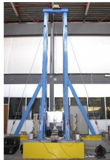
FIG. 4. ISAE-Supaero’s existing drop tower structure. The tower features an electronically operated motor and pulley system for raising test materials and two low-friction rails for keeping the test materials vertically aligned.
