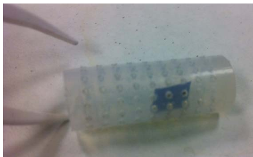
Figure 1. Photograph of a multi perforated Teflon tube containing nanostructured Ti foil.
