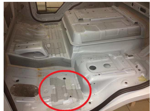
Figure 7. Upper, fibrous materials used to compose the rear panel; Lower, viscoelastic patches on the floor.
