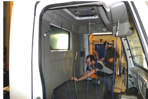
Figure 6: View of the microphones positioned inside the cabin
