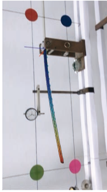
Figure 7: Three different snapshots of the raw video (left column), simulation (center) and augmented video (right). The colour map corresponds to the modulus of the displacement field.
