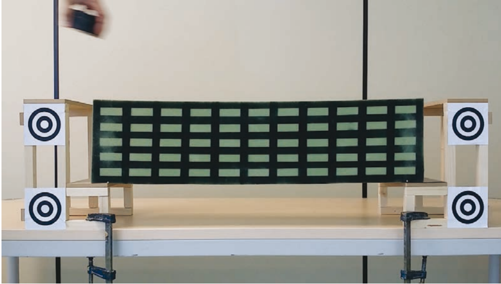
Figure 8: Geometry of the foam beam under self-weight load. This image was taken as the reference configuration of the beam. Fiducial markers were employed at this stage, that were later eliminated, to determine the pose of the camera and help to construct the reference configuration of the beam.
