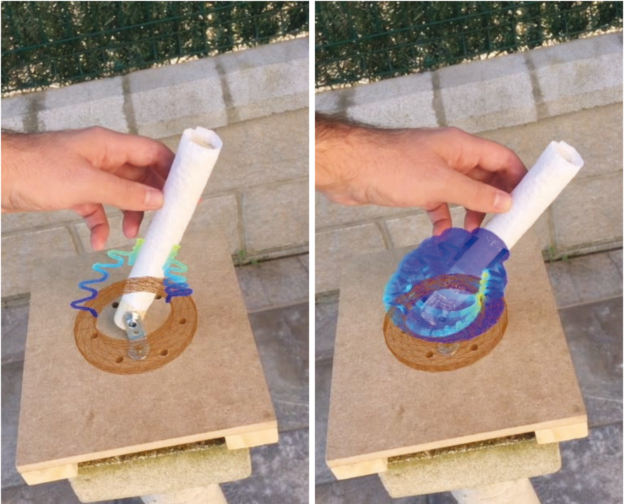
Figure 17: Two different augmented frames of the video. Color map corresponds to the modulus of the displacement field at the plane of symmetry (right) and von Mises stresses (left).
