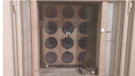
Figure 4: Glazing with retro-reflecting stickers at one side, a microphone mounted on the other side of the glass plate (traversed from one position to the other), and the loudspeaker array also on the other side of the glass plate.
