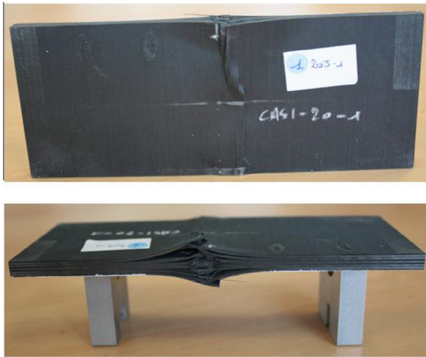
Fig. 11. CAEI failure picture of stacking 1 impacted at 20 J.
