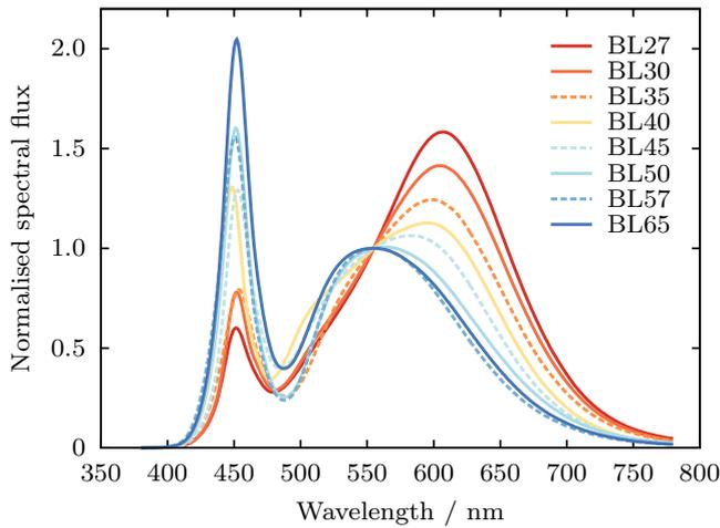
**Figure 4.** The representative spectral power distributions (RSPDs) determined from the collected LED spectra. Those five RSPDs considered to be included in the upcoming CIE technical report are shown using solid lines.
