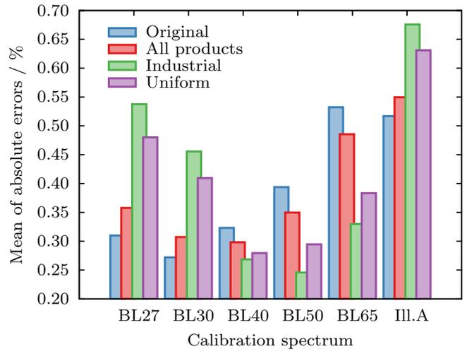
**Figure 6.** Mean absolute spectral mismatch errors produced by the five LED-based calibration spectra and Standard Illuminant A (Ill.A) for the relative spectral responsivities of the 107 photometers and the 1507 LED spectra weighted using the four distributions of figure 5.
