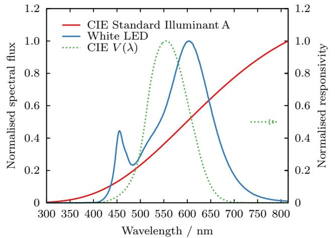
**Figure 2.** Normalised spectra of Standard Illuminant A (2856 K) and a white LED (2850 K), plotted together with  $V(\lambda)$  curve, representing the normalised spectral sensitivity of the human eye.
