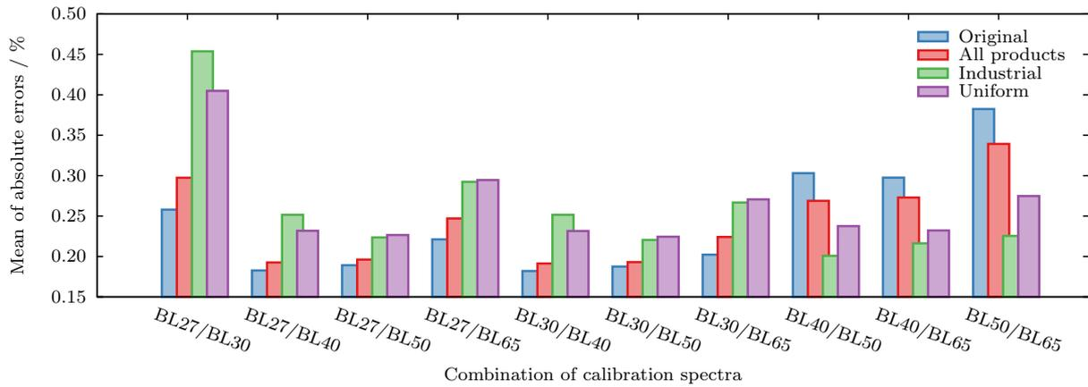
**Figure 8.** Mean absolute spectral mismatch errors produced by all combinations of the five LED-based calibration spectra for the relative spectral responsivities of the 107 photometers and 1507 LED spectra weighted using the four distributions of figure 5.
