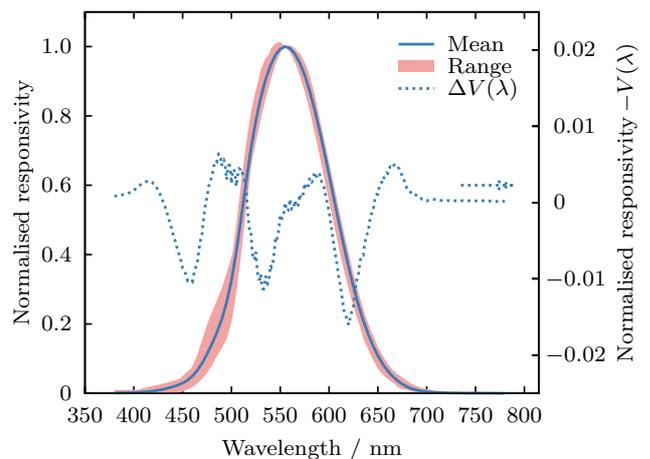
**Figure 3.** The blue solid line is the mean of the spectral responsivities of the 107 photometers used in this study. The shaded area illustrates the range of the responsivities measured for these photometers at each wavelength. The dotted line shows the difference between the mean curve and  $V(\lambda)$ .
