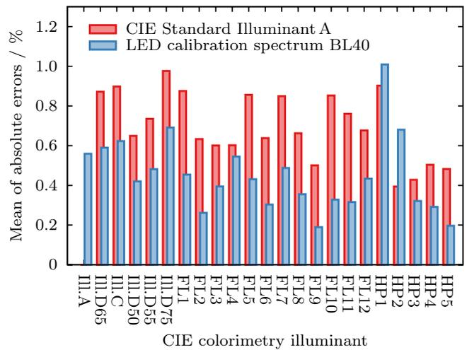
**Figure 9.** Comparison of the mean absolute spectral mismatch errors for CIE colorimetric illuminants as DUTs, when using Standard Illuminant A and LED calibration spectrum BL40 in photometer luminous responsivity calibrations.
