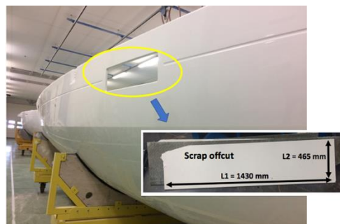
Fig. 1. Example of ship hull and trimming operation
