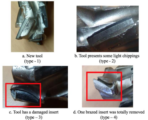
Fig. 6. Four types of the tool condition
