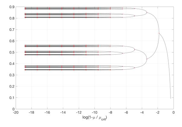
Figure 1: Bifurcation diagram of the logistic map obtained with Manlab 4.0. The red dots are period doubling bifurcations. The x-axis is  $\log(1 - \frac{\mu}{\mu_{\text{crit}}})$  where  $\mu_{\text{crit}}$  is the critical value above which the system becomes chaotic. The 12 first bifurcations were computed.
