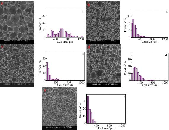
**Fig. 3.** SEM and cell size distribution of (a) DE foam with density 32 kg/m<sup>3</sup>; (b) DE foam with density 62 kg/m<sup>3</sup>; (c) DE foam with density 87 kg/m<sup>3</sup>; (e) pentane foam with density 120 kg/m<sup>3</sup>; (f) DEP foam with density 100 kg/m<sup>3</sup>
