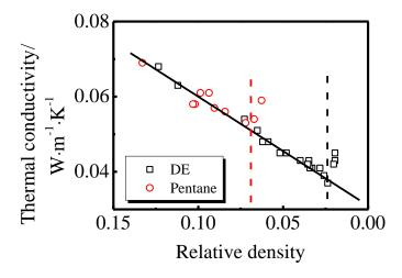
**Fig. 5.** Effect of relative density of tannin/furanic rigid foam on thermal conductivity. The straight line fits the linear region of DE foam.
