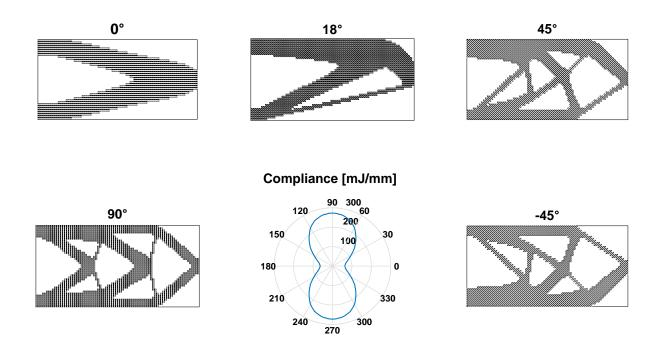
Fig. 1: Optimal compliance with respect to material orientation in a polar representation (middle, bottom) and five optimal shapes corresponding to 0° (left, top), 18° (middle top), 45° (right, top), 90° (left, bottom) and -45° (right, bottom) material uniform orientations of the cantilever beam problem made of long and straigth carbon fibers in an epoxy matrix (left side of the structure is clamped, a vertical load is applied in the middle of the right side).
