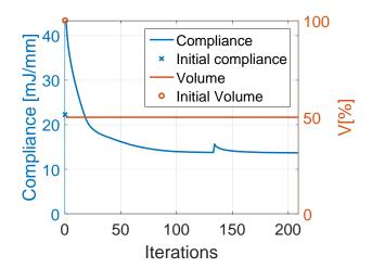
Fig. 4: Compliance and volume with respect to optimization iterations
