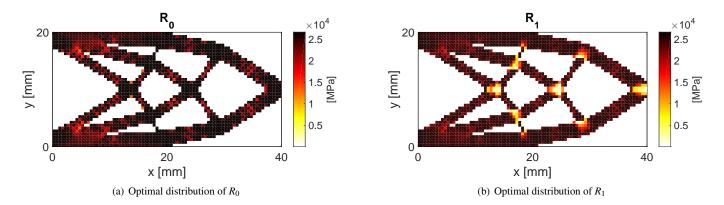
Fig. 7: Optimal distribution of the stiffness tensor anisotropic polar invariants
