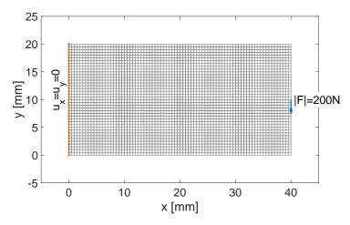
Fig. 3: Boundary conditions for the Cantilever beam optimization problem
