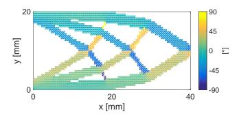
Fig. 6: Optimal distribution of orthotropy direction
