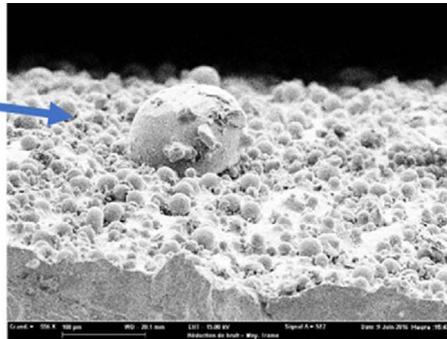
Fig. 7. Non-melted particle ( $D \approx 100 \mu\text{m}$ ) on a SLM surface (a) 3D scan and (b) SEM image.
