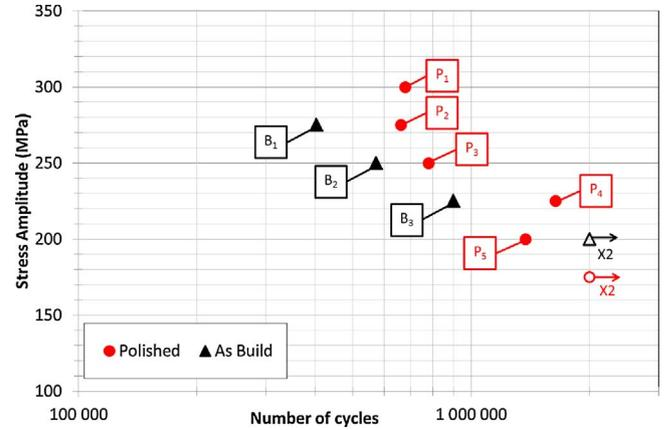
Fig. 12. S-N curves for polished and as-built batches.
