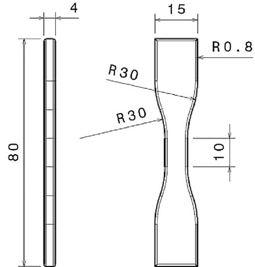
Fig. 3. Geometry of the specimens tested in fatigue.
