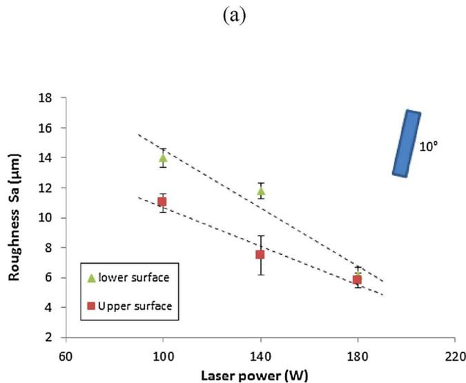
Fig. 5. (a) Average roughness Sa measured on bottom and top surfaces for  $\theta = 10^\circ$  building angle, (b) SEM image for  $P = 140\text{W}$ ,  $V = 0.5\text{ m/s}$  (sample 2, upper side), (c) SEM image for sample 2 (lower side).
