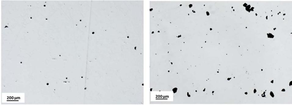
Fig. 11. 2D quantification of the voids fraction a) in the cross-section (0.3% of spherical porosities) b) close to the surface (2.2% of porosity) (sample 24: 150 W-0.6 m/s-10°).
