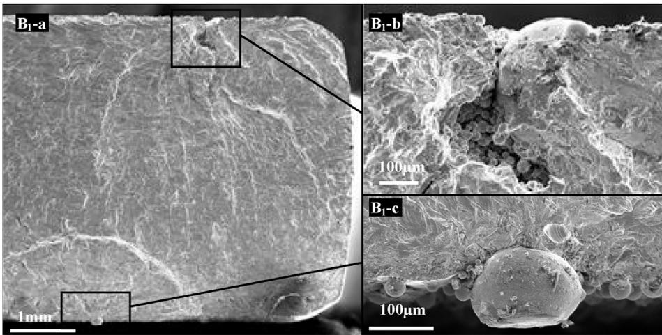
the surface scan using the fracture surface analysis. Fig. 15 shows the surface scan and a close-up of the critical defect of the as-built specimen B<sub>3</sub>.
