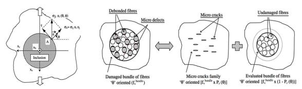
Fig. 3. (a) Projection of the stress tensor (normal and shear interface stresses,  $\sigma$  and  $\tau$  respectively). (b) Micromechanical damage description. (From Jendli & al. [27]).
