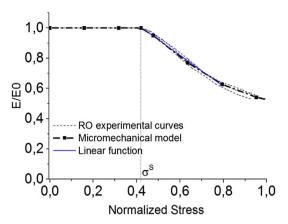
Fig. 4. Evolution of the relative loss of stiffness during tensile loading
