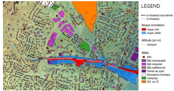
Fig. 7: Map of the flood risk (red or high risk and blue for low risk) in Roubaud valley.
