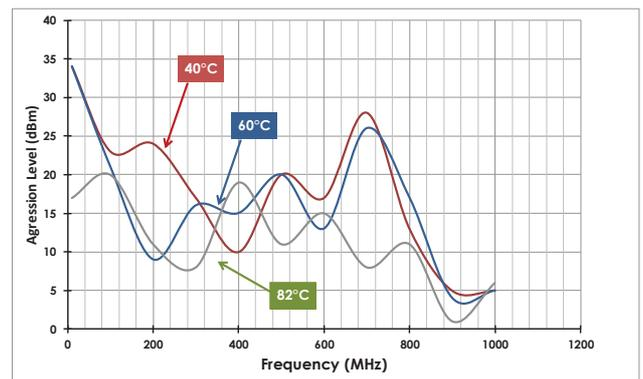
Fig. 8. Immunity table at temperature steps of 20°C for criteria "1%" on duty cycle  $\alpha$
