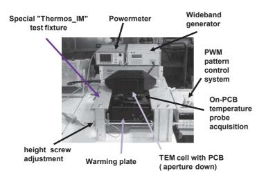
Fig. 6. View of the heated TEM-Cell configuration for immunity testing.
