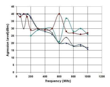
Fig. 7. Immunity table reference(20°C) for the four criterias:  $\diamond$  duty cycle  $\alpha$   $\Box$  frequency jitter  $\Delta$  Switching margins  $V_{MEAN}$
