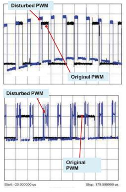
Fig. 3. Views of signal shifts on nominal PWM waveforms during harmonic aggression.
