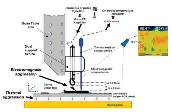
Fig. 1. Schematic of the experimental dual thermal-near field set-up configuration for immunity testing on conventional PCB.
