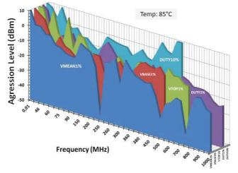
Fig. 9. 3D table representation of worst-case's immunity with PCB temperature of 85°C, for 5 criterions of the PWM: Duty10%, Duty1%, Vtop1%, Vbase1%, Vmean1%
