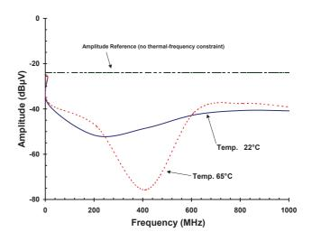
Fig. 5. Relative variation of switching amplitude of Integrated PWM circuit with dual thermal-harmonic wave aggressions
