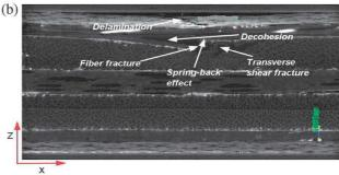
**Fig. 8.** Tomography images of impacted plywood with glass skins – Failure modes at 15 J, (a) plywood A, (b) plywood B. (For interpretation of the references to colour in this figure legend, the reader is referred to the web version of this article.)
