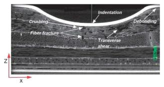
**Fig. 5.** Tomography images of impacted plywood with aluminum skin – Failure modes at 15 J. (For interpretation of the references to colour in this figure legend, the reader is referred to the web version of this article.)
