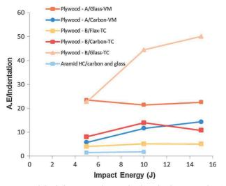
**Fig. 11.** Ratio of absorbed energy to indentation for plywood with composite skins (J/mm). (For interpretation of the references to colour in this figure legend, the reader is referred to the web version of this article.)
