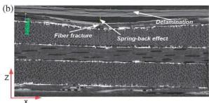
**Fig. 7.** Tomography images of impacted plywood with Carbon skins – Failure modes at 15 J, (a) plywood A, (b) plywood B. (For interpretation of the references to colour in this figure legend, the reader is referred to the web version of this article.)
