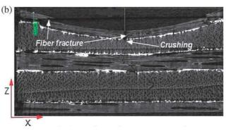
**Fig. 3.** Failure modes of impacted plywood core at 10 J. (a) Plywood A, (b) Plywood B. (For interpretation of the references to colour in this figure legend, the reader is referred to the web version of this article.)
