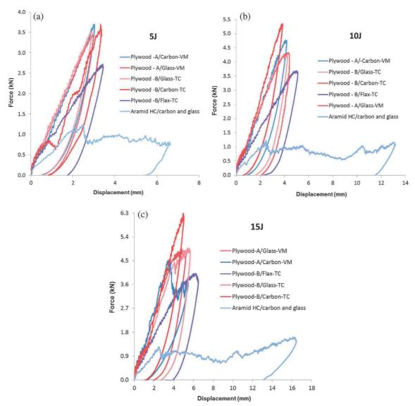
Fig. 10. Force displacement plot for Sandwich panels with plywood core and composite skins at 5 J (a), 10 J (b), 15 J (c). (For interpretation of the references to colour in this figure legend, the reader is referred to the web version of this article.)
