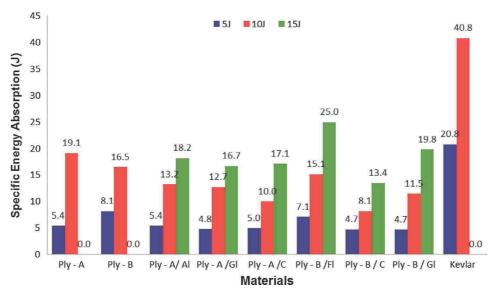
Fig. 13. Specific energy absorption for the 8 configurations tested plus the reference one. (For interpretation of the references to colour in this figure legend, the reader is referred to the web version of this article.)
