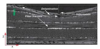
**Fig. 9.** Tomography images of impacted plywood with flax skins – Failure modes at 15 J, plywood B. (For interpretation of the references to colour in this figure legend, the reader is referred to the web version of this article.)
