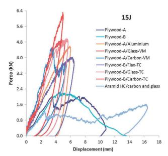
**Fig. 12.** Force-displacement plot for the different wood based sandwich structures at 15 J. (For interpretation of the references to colour in this figure legend, the reader is referred to the web version of this article.)
