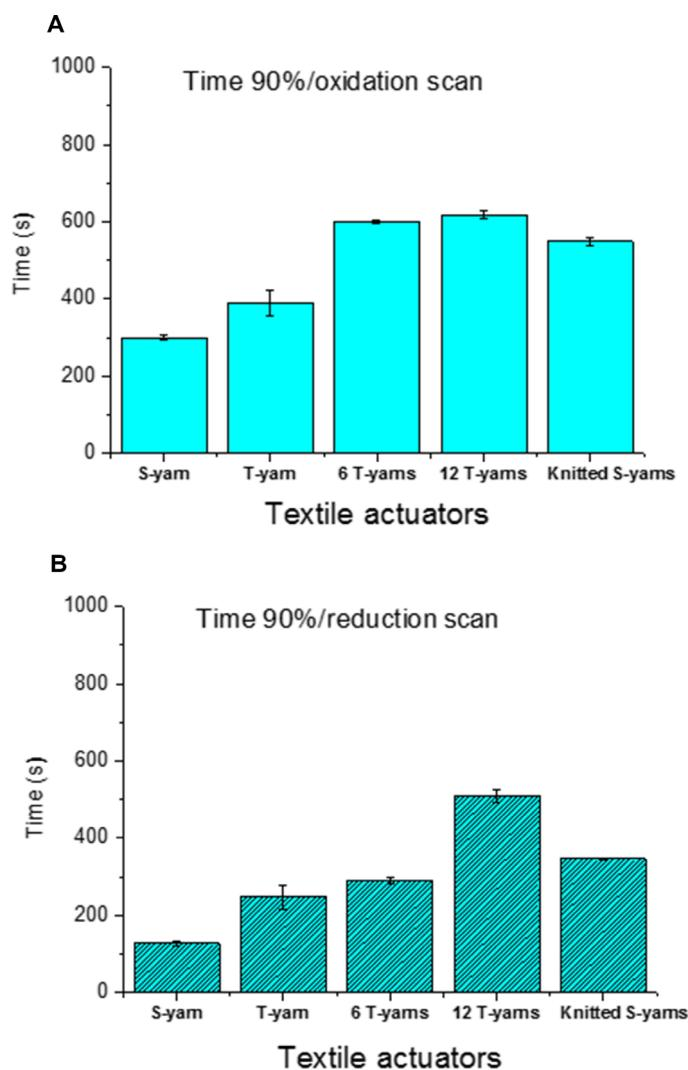
**Fig. 4. Evaluation of the actuation speed for the textile actuators.** Time to 90% maximum contraction (oxidation scan) and elongation (reduction scan) for individual S-yarn, individual T-yarn, 6 T-yarn weave, 12 T-yarn weave, and knitted S-yarns during activation between 0.5 and  $-1$  V for 800 s.
