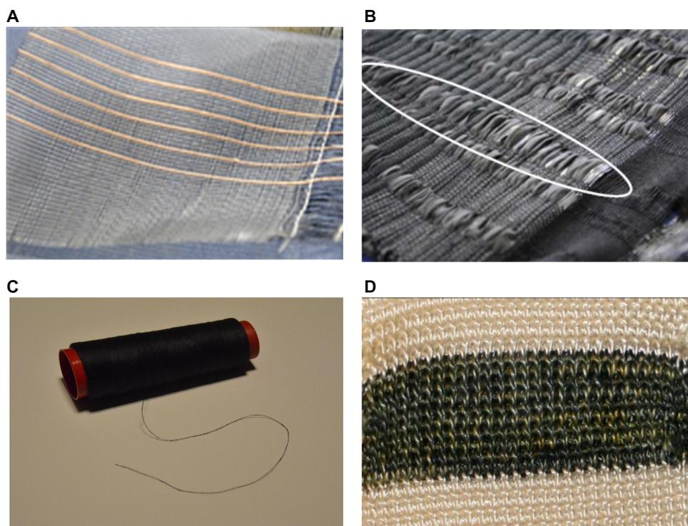
**Fig. 11. Processing and integration of electroactive textiles.** (A) Cu monofilaments in weave fabric. (B) Example of a custom weave with spacing (marked) that enables movements of yarns within the marked area. (C) A bobbin with industrially manufactured PEDOT-coated yarn. (D) A knitwear structure for respiratory monitoring comprising CP-coated yarns (black yarn) knitted together with normal (white) yarn.
