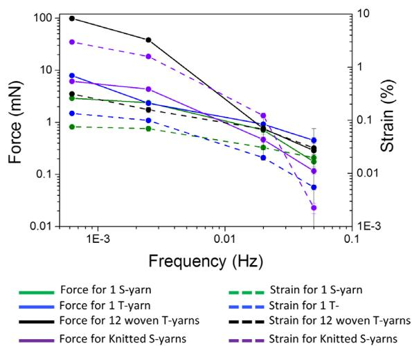
**Fig. 9. Frequency response of the textiles actuators.** Measured isometric force and isotonic strain ( $\Delta L/L_0$ ) versus frequency for individual S-yarn, individual T-yarn, 12 T-yarn weave, and knitted S-yarn during activation of the actuators between 0.5 and  $-1$  V for 800, 200, 25, and 10 s, average of five measurements.
