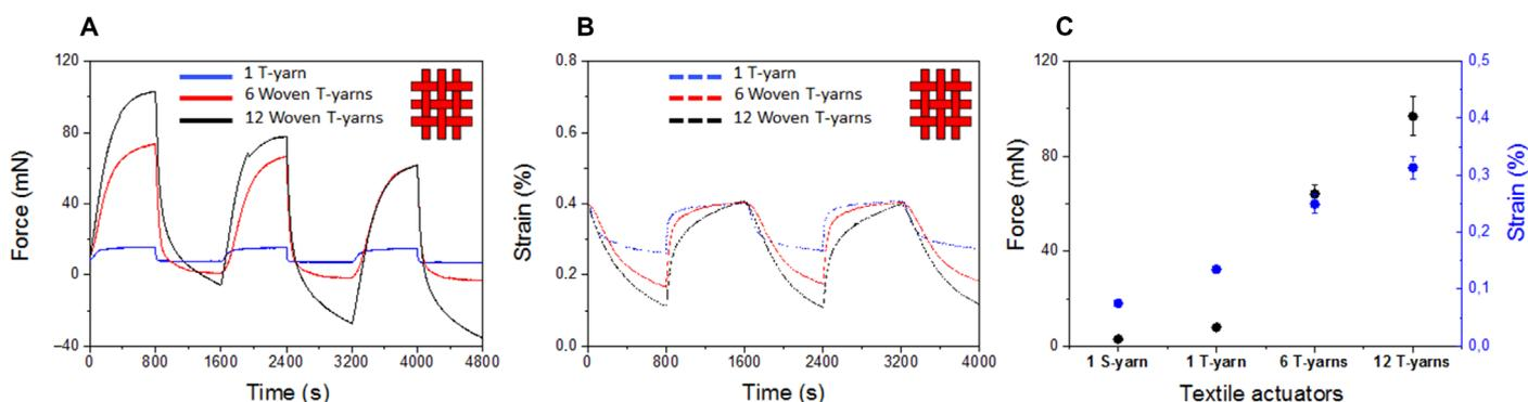
**Fig. 3. Electromechanical characterizations of the woven textile actuators.** (A) Measured isometric force and (B) isotonic strain ( $\Delta L/L_0$ ) versus time for individual T-yarn, 6 T-yarn weave, and 12 T-yarn weave during activation between 0.5 and  $-1$  V for 800 s. (C) A comparison between the measured isometric force and the isotonic strain of the individual yarns, 6 T-yarn weave, and 12 T-yarn weave as average of five measurements.
