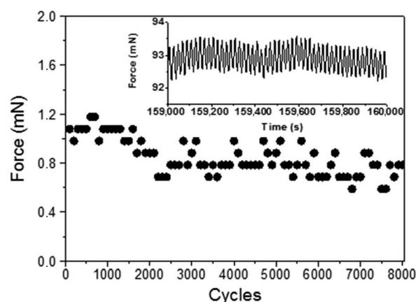
**Fig. 5. Life cycle test of the woven textile actuators.** Life cycle test of 12 T-yarn weave during activation between 0.5 and  $-1$  V for 10 s for 44 hours. Insert: Measured force versus time of the last 50 cycles of the life cycle test.
