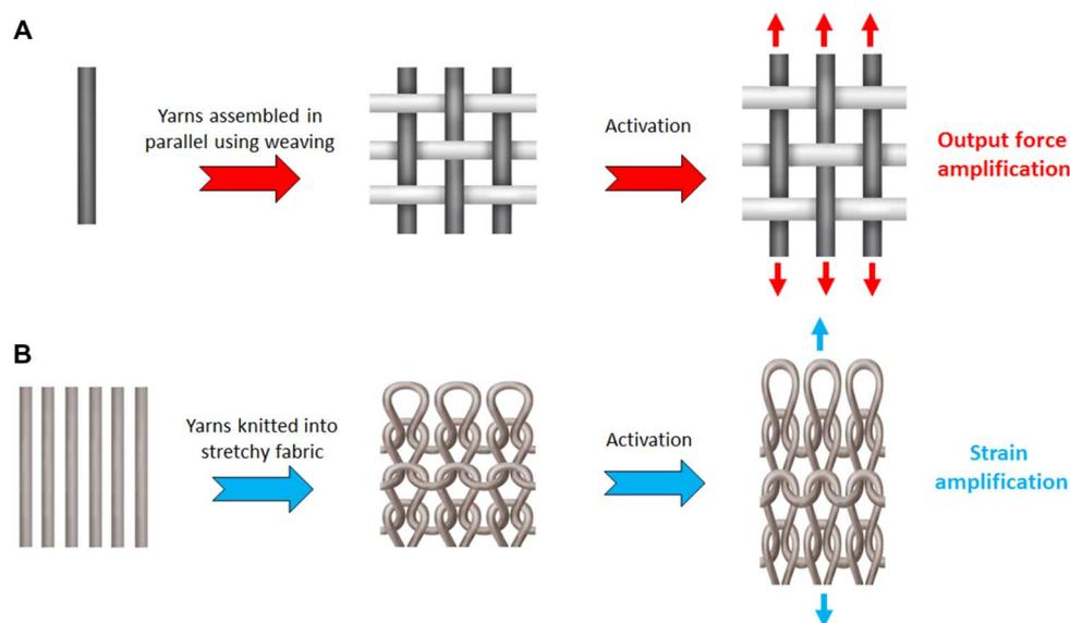
**Fig. 1. Concept of the textile actuators (textuators).** (A) The textuators scale up force by weaving of single yarns in parallel. (B) The textuators amplify the strain by using stretchable knitted patterns.
