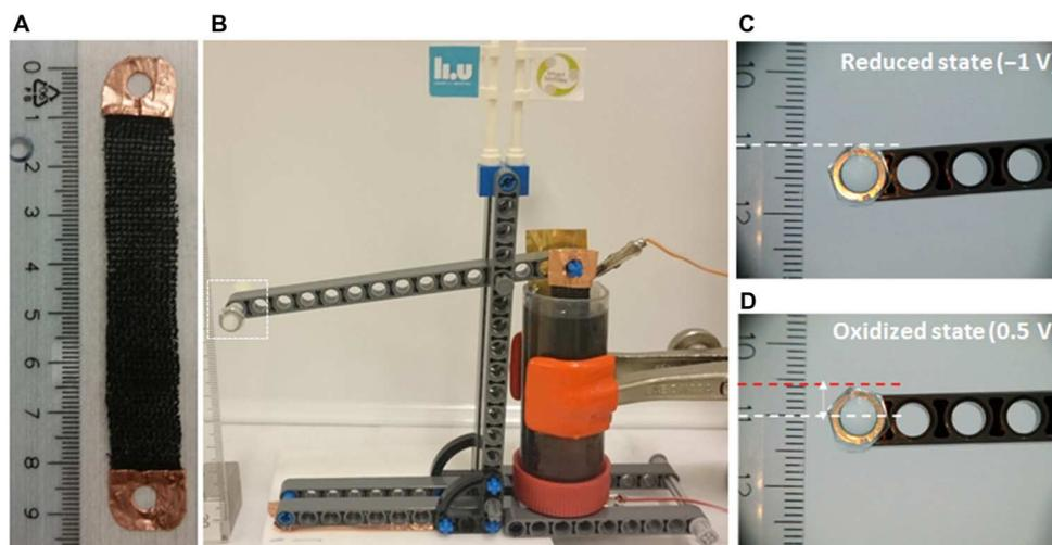
**Fig. 10. Applications of the textile actuators.** (A) A knitted textuator unit. (B) The textuator unit (~3-cm active length) drives a lever arm in a LEGO setup. The arm lifted a 2.0-g load when switched between  $-1$  (reduced state, C) and  $0.5$  V (oxidized state, D).
