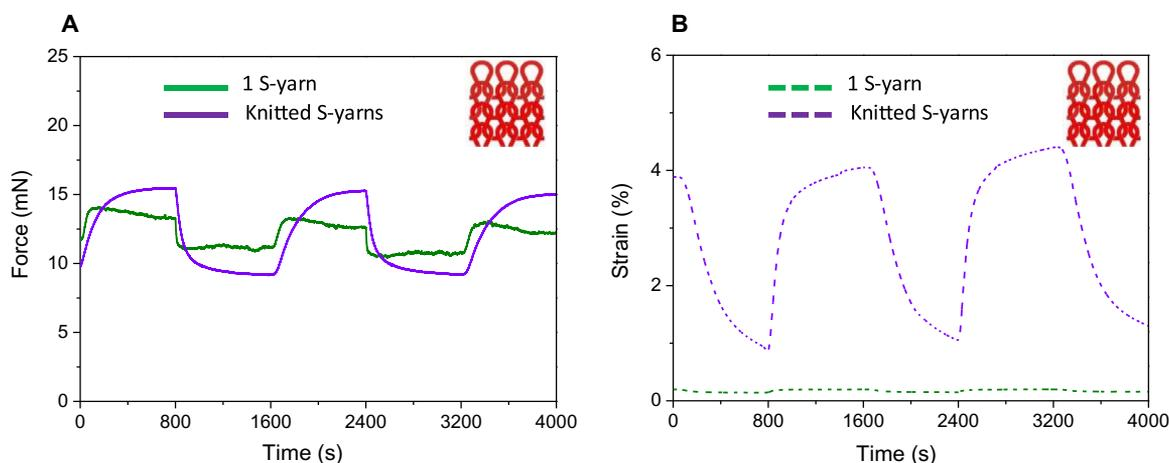
**Fig. 6. Electromechanical characterizations of the knitted textile actuators.** Measured (A) isometric force and (B) isotonic strain ( $\Delta L/L_0$ ) versus time for S-yarn and knitted S-yarn fabric during activation between 0.5 and  $-1$  V for 800 s.
