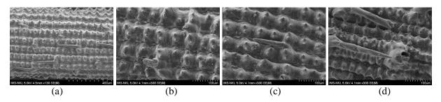
Figure 5. SEM images of surface of RH and its chars. (a): RH, (b):  $600^{\circ}$ C,  $20.min^{-1}$  char, (c):  $900^{\circ}$ C,  $20.min^{-1}$  char and (d):  $900^{\circ}$ C,  $1800^{\circ}$ C.min<sup>-1</sup> char
