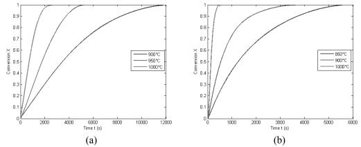
**Figure 6.** Influence of reaction temperature on char conversion (a) under CO<sub>2</sub> and (b) under H<sub>2</sub>O atmosphere (Partial pressure of the reacting gas: 0.2 atm)
