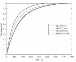
**Figure 8.** Influence of HR on char conversion (H<sub>2</sub>O partial pressure: 0.2 atm, temperature: 900°C)
