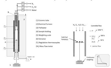
Figure 4. Macro-thermogravimetric reactor and its principle
