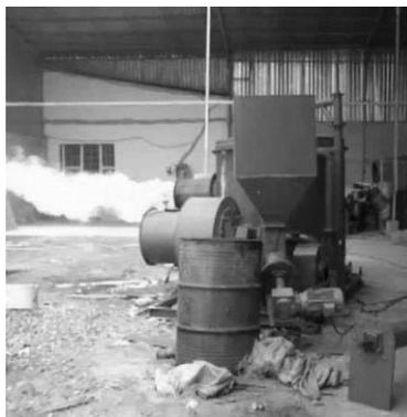
**Figure 2:** A RH gasifier for heat generation (Source: <https://hayvip.com>)
