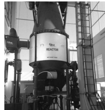
Figure 3: RH gasifier for power generation in Cambodia (Picture taken by author)
