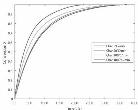
**Figure 8.** Influence of HR on char conversion ( $\text{H}_2\text{O}$  partial pressure: 0.2 atm, temperature:  $900^\circ\text{C}$ )
