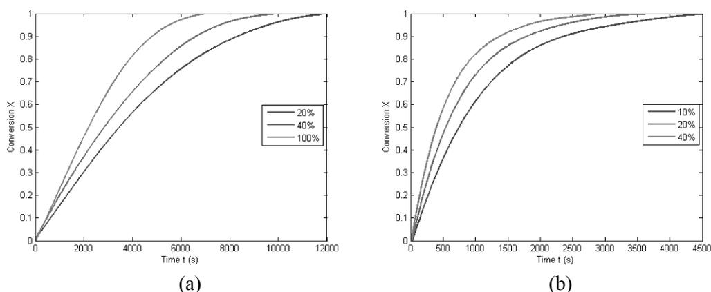
**Figure 7.** Influence of partial pressure of reacting gas on char conversion (a) under CO<sub>2</sub> atmosphere and (b) under H<sub>2</sub>O atmosphere (Temperature of reacting gas: 900°C)
