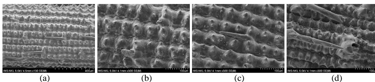
**Figure 5.** SEM images of surface of RH and its chars. (a): RH, (b): 600°C, 20.min<sup>-1</sup> char, (c): 900°C, 20.min<sup>-1</sup> char and (d): 900°C, 1800°C.min<sup>-1</sup> char
