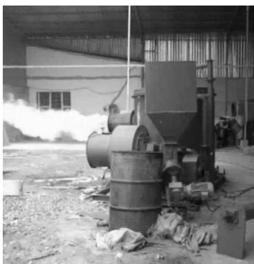
Figure 2: A RH gasifier for heat generation (Source: https://hayvip.com )
