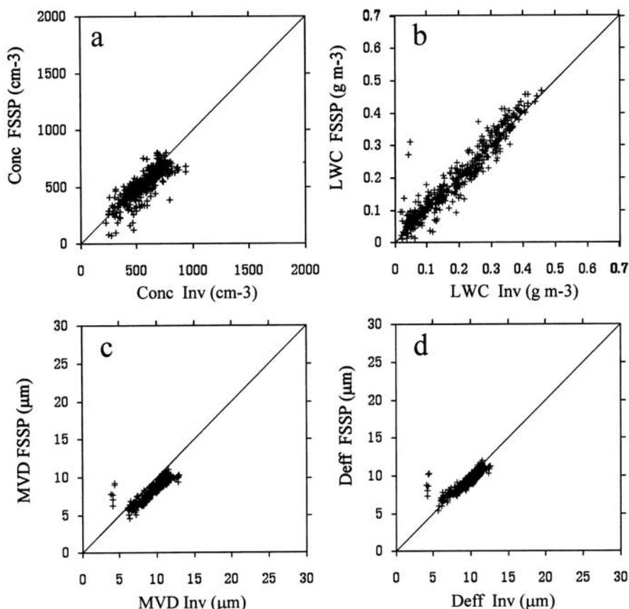
**Figure 3.** (a–d) Comparison of direct (FSSP) and retrieved (Polar Nephelometer) microphysical parameters (Conc, cloud droplet concentration; LWC, liquid water content; MVD, mean volume diameter; Deff, effective diameter). The results concern the water droplet cloud sequence for the stratocumulus cloud observed on 21 January 1999.
