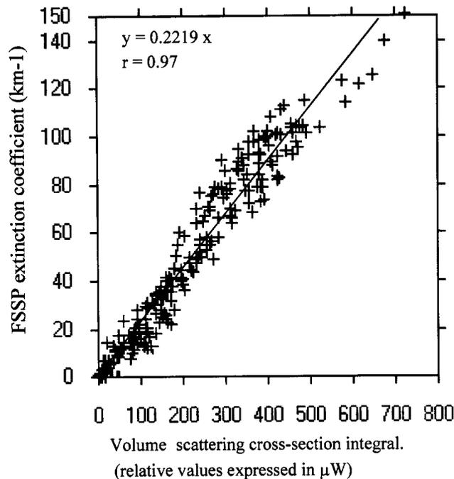
**Figure 4.** Visible extinction coefficient derived from the FSSP measurements versus the relative values from the integral (from  $15^\circ$  to  $155^\circ$ ) of the scattering cross-section measured by the Polar Nephelometer.
