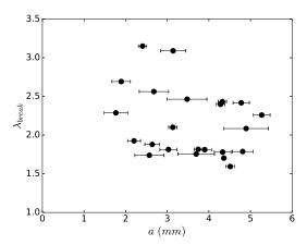
Fig. 15 Natural rubber stretch at break with respect to notch initial length for small length notches
