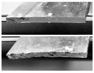
Fig. 8 Unfilled SBR surfaces created after crack propagations: smooth shiny surface for initial small cut (top) and rough surface for initial large notch (bottom).
