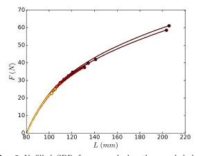
Fig. 9 Unfilled SBR force-sample length recorded during uniaxial tension for specimens with initial notches varying between 500  $\mu$ m to 5 mm. The circles indicate the elongations at break. Light colors correspond to the longer notches.
