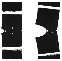
Fig. 6 Comparison of the SENT specimen states of deformation during applied uniaxial tension for a small notch (left) and a large notch (right) filled SBR samples.
