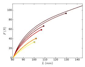
Fig. 5 Filled SBR force-sample length recorded during uniaxial tension for specimens with initial notch larger then 6 mm. For reference, the top line shows the response of a specimen with a small notch. Lighter colors correspond to the longer initial notches. Circles mark the sample breaks.
