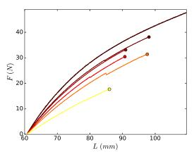
Fig. 16 Natural rubber force-sample length recorded during uniaxial tension for specimens with initial notch larger then 5 mm. The top curve shows the behavior of a sample presenting a small notch. The circles indicate the elongations at break. Light colors correspond to the longer notches.
