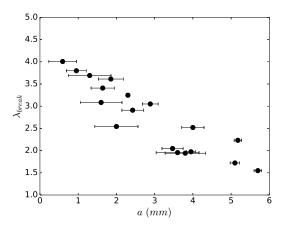
Fig. 4 Filled SBR stretch at break with respect to notch initial length extracted from figure 2 for small length notches.
