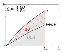
${f Fig.~1}$  Fragile fracture Griffith analysis at constant applied elongation.
