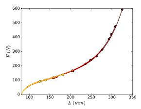
Fig. 2 Filled SBR force-sample length recorded during uniaxial tension for specimens with initial notches varying between 500  $\mu$ m to 6 mm. The circles indicate the elongations at break. Light colors correspond to the longer notches.
