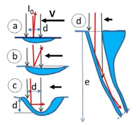
FIG. 1. (a-d) As a function of the welding speed V, evolution of the melt pool geometry leading to the KH formation.
