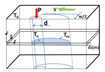
FIG. 2. Sketch of the longitudinal section of an inclined keyhole. The incident beam power is P. The KH surface is  $T_v$  and its diameter is d. The width of the melting isotherm  $T_m$  is w. Welding speed is V.
