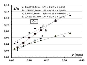
FIG. 6. For Cu and different operating parameters, plot of 1/R as a function of the welding speed V and corresponding best linear fits.
