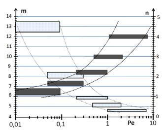
FIG. 4. Inside five selected Pe intervals, ranging from Pe = 0.01 to Pe = 10, mean values of the pair of parameters m (empty symbols) and n (filled symbols) used for defining the corresponding best fit for a linear variation of g(Pe), as g(Pe) = mPe + n.
