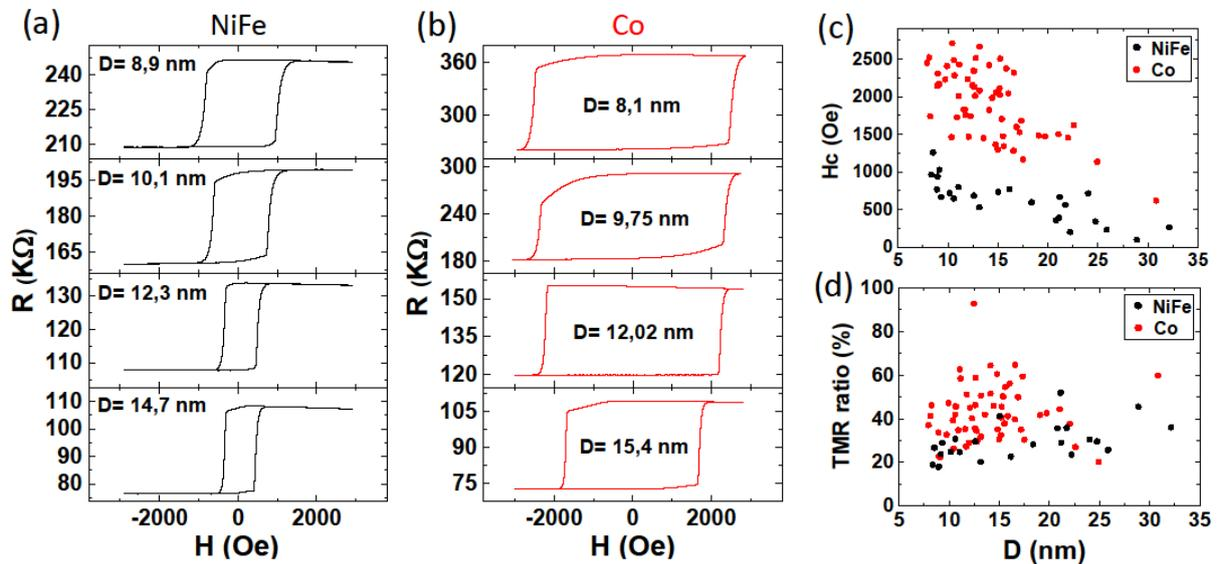
**Fig. 4.** (a), (b) Evolution of the resistance  $R$  as a function of a perpendicular field for MTJ of various diameters  $D$  in the cases of a 60 nm thick storage layer of NiFe and Co respectively. (c) Distribution of coercive fields  $H_c$  as a function of  $D$  for NiFe (black circles) and Co (red circles) storage layer. (d) Distribution of the TMR ratio as a function of  $D$  for NiFe (black circles) and Co (red circles) storage layer.
