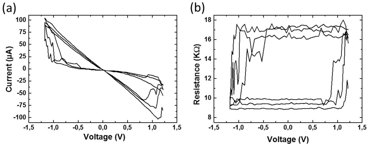
**Fig. 5.** Evolution of current (a) and resistance (b) versus applied voltage at zero external field. illustrating STT switching in a PSA-MTJ with 12 nm thick FeCoB(2)/CoFeB(8)/FeCoB(2) free layer, with a MgO capping layer on top, and a diameter of 17 nm.
