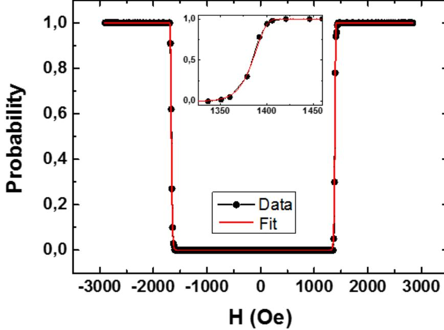
**Fig. S1.** Evolution of the probability of switching ( $P_{\text{sw}}$ ) as a function of the perpendicular applied field, determined from the switching field distribution obtained after 300 RH loops at a fixed field sweep rate of 5.4 kOe/s. Black line with circle symbols represents the data. Red solid line shows the fit according to eq.8. In inset is shown a zoom on the transition from P to AP states.
