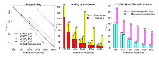
FIG. 7. Left: Strong scaling for 512<sup>3</sup> synthetic particles and grid sizes ranging from 1024<sup>3</sup> to 8192<sup>3</sup>. Center: Scaling of individual tessellation and density estimation components. Right: Comparison of 2D and 3D output for 512<sup>3</sup> synthetic particles and 1024<sup>3</sup> grid.
