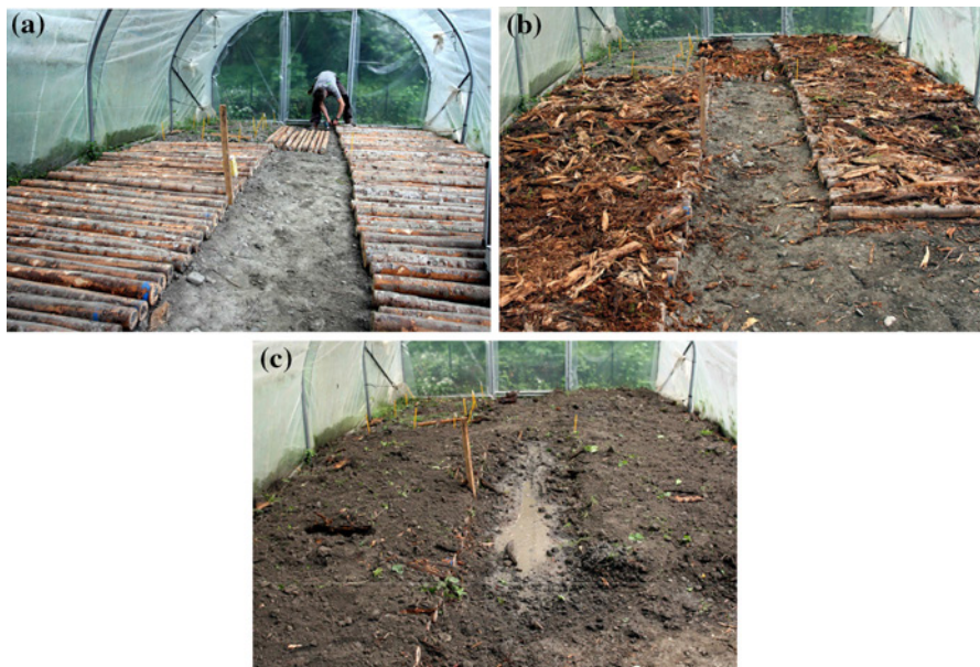
Fig. 1 Successive steps of sample preparation in the greenhouse: a The small-diameter logs laid on the ground. b The small-diameter logs covered by woody debris. c Samples covered by a local soil layer
