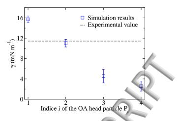
Figure 4: Interfacial tension of the water–OA mixture (system 9) versus the index i of the carboxylic acid polar bead  $P_i$ . The higher the index i, the higher the polarity of the bead.
