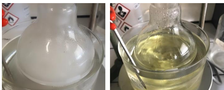
Figure 1 Mixture of tin hydroxide with acetic acid and ethylene glycol before heating (left); after heating (right) at 90^\circ\text{C}
