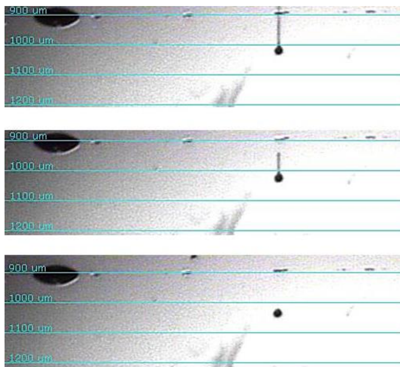
Figure 5 Strobe photographic images showing an ejected drop of SnO 2 ink
