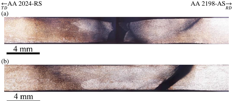
Figure 4. Fracture locations after monotonic tensile tests found in the middle of the joint or on the advancing side in the TMAZ. a) tool F, b) tool G.
