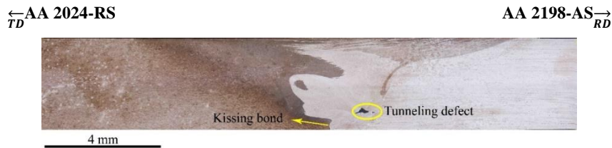
Figure 7. Cross-sectional observations of joint produced by tool F at 750 rpm and 450 mm/min welding speed which contain tunneling and kissing bond defects.
