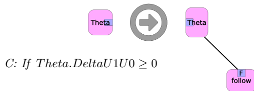
Fig. 9. Follow Result. Applies if \text{DeltaU1U0} \geq 0 . As additional visualisation support, it generates a follow node, which indicates that it is more profitable to follow the negligence rule and not do a full risk analysis
